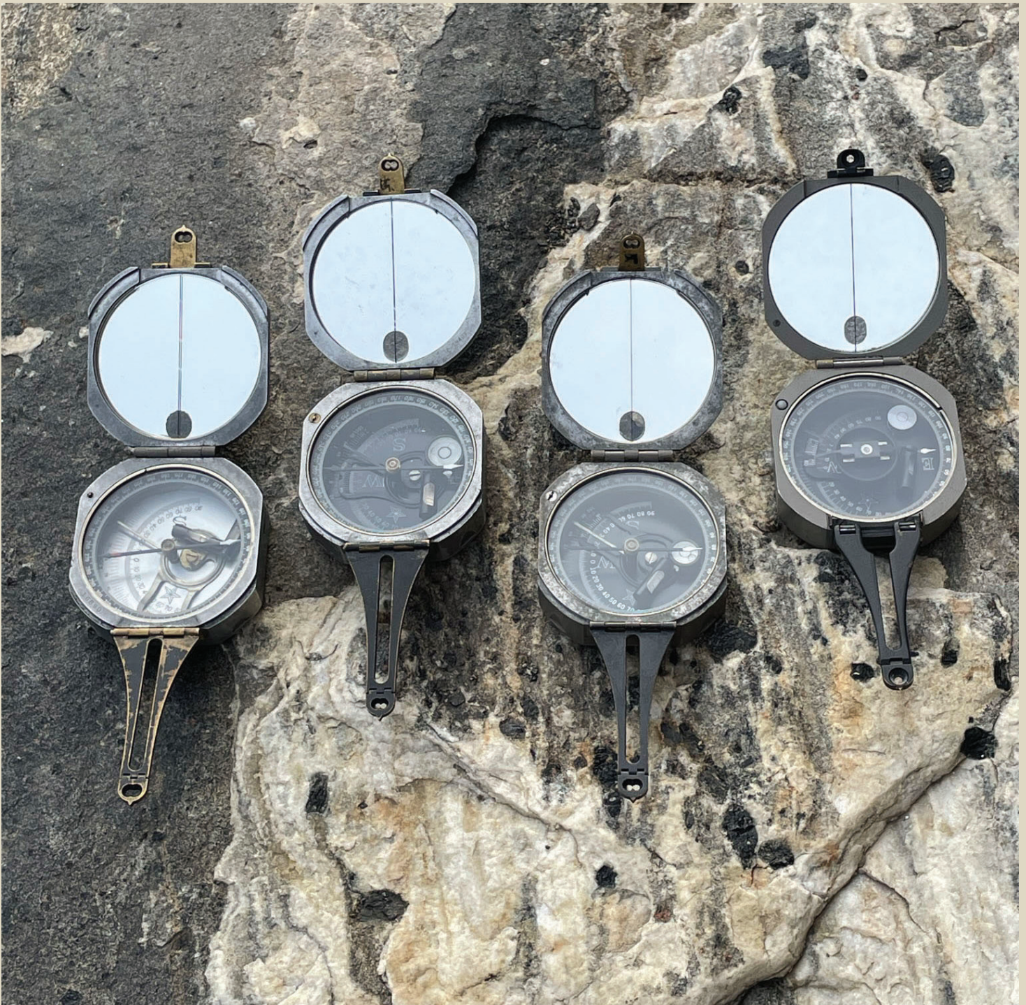
A selection of Brunton compasses used to teach generations of U of T geoscience students since the 1920's. Photo by Heidi Tomes.
